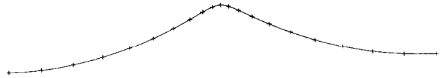
FIG. 2. Propagation of a steep steady periodic wave of amplitude ak = 0.42 using 20 points. The initial continuous surface is shown as well as the surface points (marked +) after five wave-periods (natural scale).
